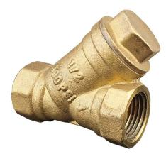
Profit brass strainers can serve in piping systems that are sensitive for any debris in the medium. They filter out solid parts to protect other equipment such as alarm valves from damage or bad functioning. Type DYST-1/2 has female threaded ends. The strainers are designed so that they can be cleaned without removing them from the piping system.
