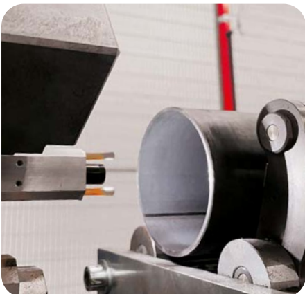
Automatic pipe seam detection & positioning
